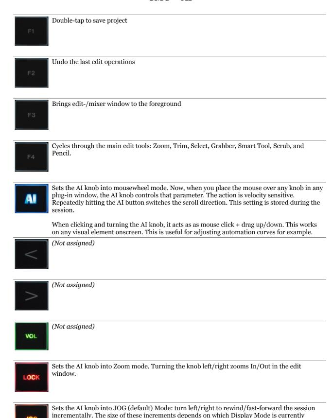
Repeatedly hitting the JOG button switches between the default JOG and alternative JOG Mode: turn left/right to move the cursor to the previous or next clip- (region) boundary. The
