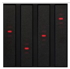
Volume/Send level faders. By default the faders controls the volume faders 1-4 within the HUI faderbank. When a second CMC-FD unit is connected to CMC-FD: port 2, this unit controls the volume faders 5-8 within the HUI faderbank.
